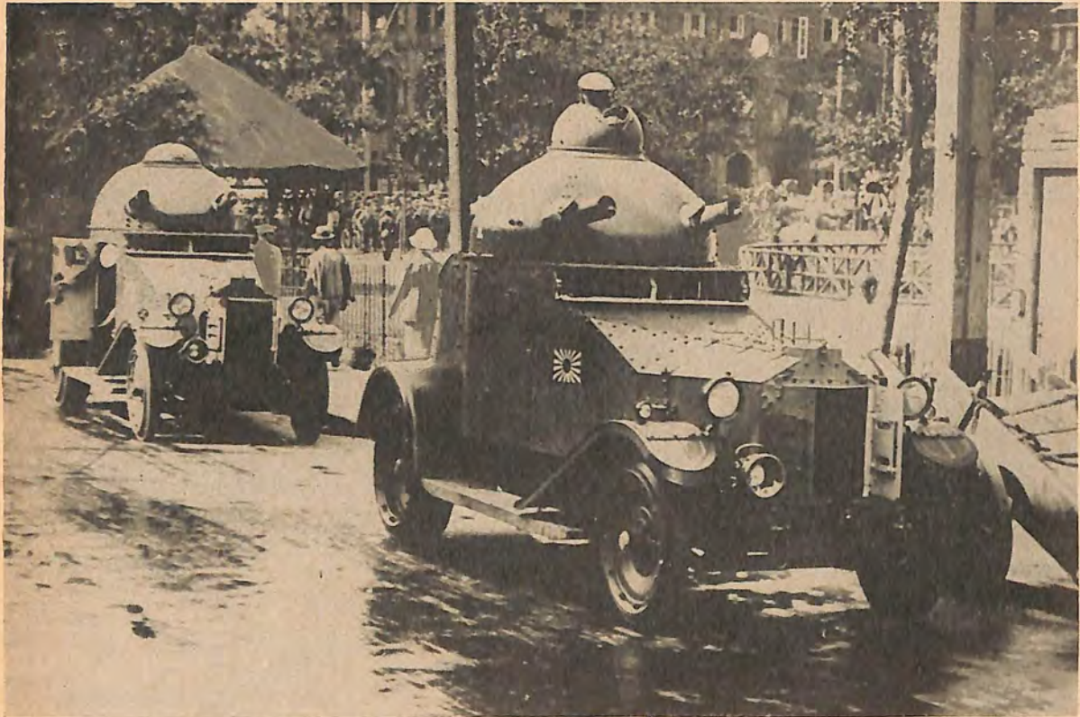
Figure 251. Model 25 (?) "Vickers Crossley" armored car.
